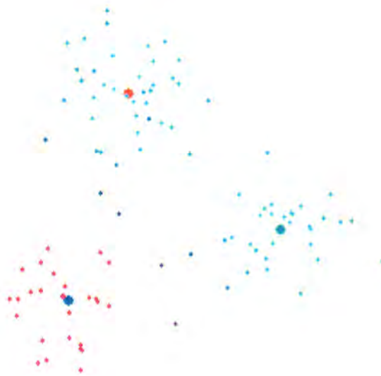
Figure 2. A snapshot of the grand tour view of the fuzzy c-means clustering algorithm. The data points are colored according to their membership in the blue (lower left) cluster, with red representing high membership and light blue representing low membership.
